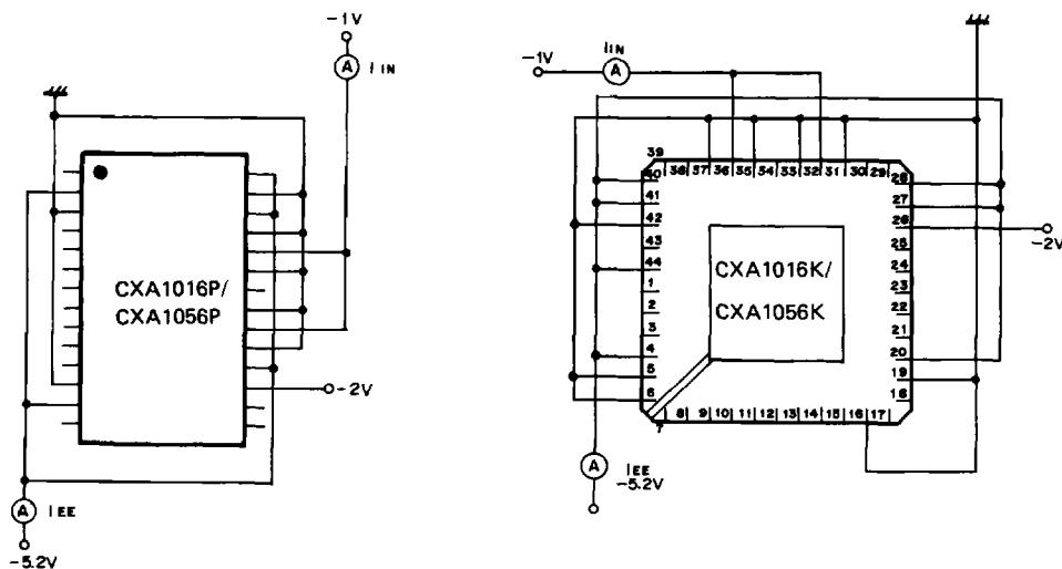
**Aperture Jitter Test Circuit**
