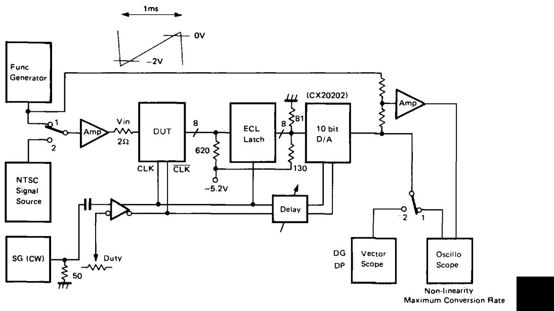
**Differential Non-linearity Test Circuit****Integral Non-linearity Test Circuit**
