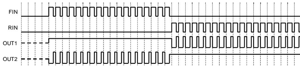
Fig.17 PWM control operation (timing chart)
