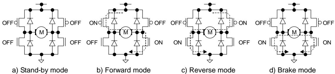
Fig.15 Four basic operations (output stage)
