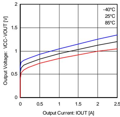
Fig.10 High side body diode
