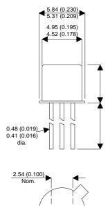
ტ 3 Bipolar NPN Device in a Hermetically sealed TO18 Metal Package.
