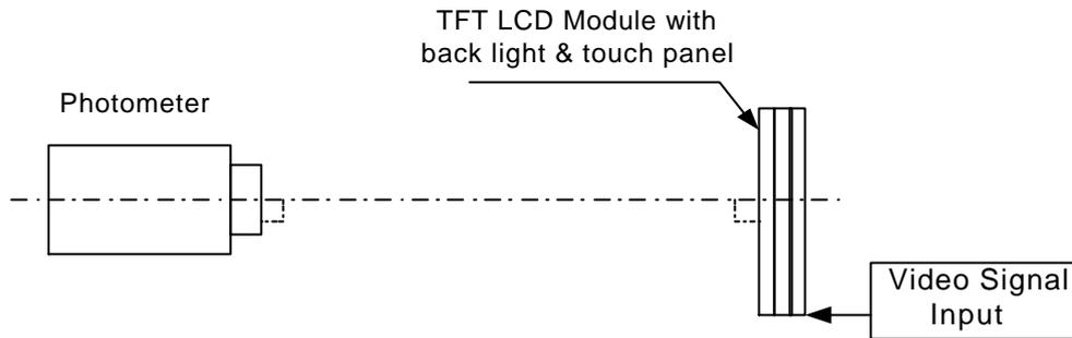
Note 9-1: Viewing angle diagrams (Measure System B)
