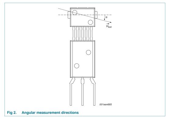
Since the Anisotropic MR (AMR) effect is periodic over 180°, the sensor output is also 180°-periodic, where the angle is calculated relative to a freely programmable zero angle. The dashed line indicates the mechanical zero degree position.
