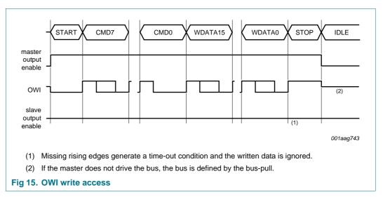
**Note**: As already mentioned in <u>Section 13.1</u>, the command mode has to be entered using the write procedure. If command mode is not entered, communication is not possible and the sensor operates in normal operation mode. After changing an address, the time  $t_{prog}$  must elapse before changing another address. Finally the checksum must be recalculated and written, because the contents of the non-volatile memory have been changed (see <u>Section 13.4</u>).
