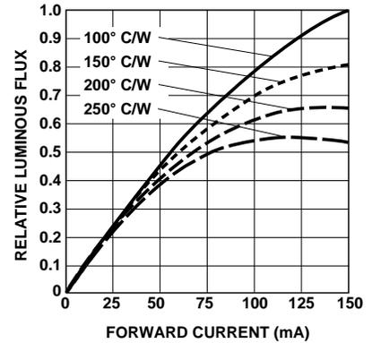
Figure 4. HPWS-xx00 Relative Luminous Flux vs. Forward Current.
