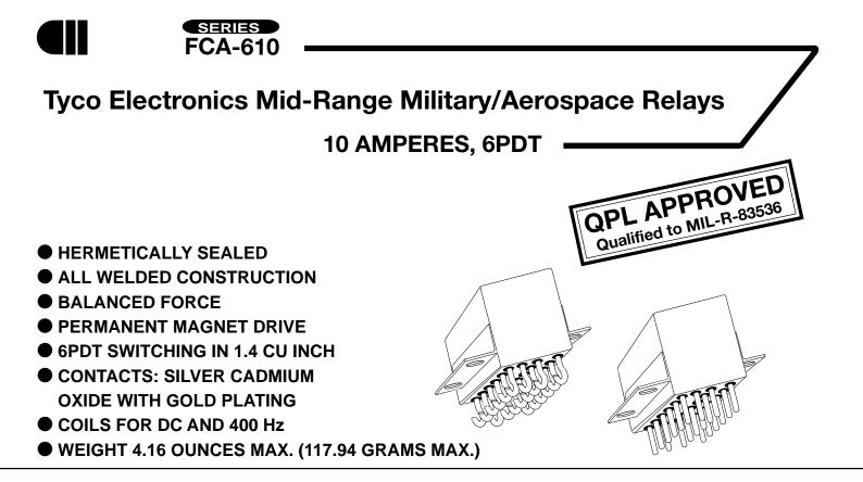
The Series FCA-610 relay is a polarized single-side stable design, where the flux from a permanent magnet provides the armature holding force in the deactivated state, and its flux path is switched and combined with the coil flux in the operated state. This results in appreciably increased contact pressure in both states over that of a spring return nonpolar design. We also manufacture 2-pole and 4-pole versions of this relay.
