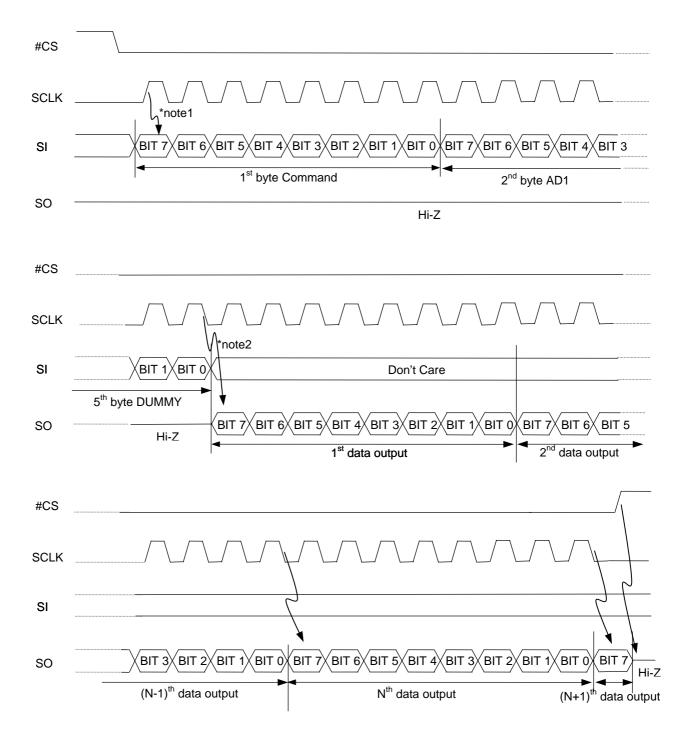
Fast Read Array Timing Waveform
