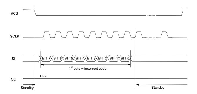
Incorrect command makes this LSI become and keep standby mode until next #CS rising edge. In standby mode, SO pin is High-Z.
