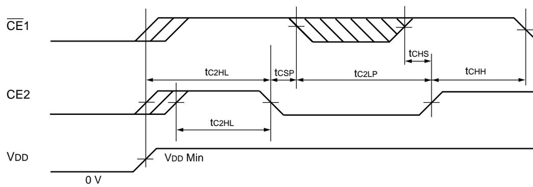
Note : The  $t_{C2HL}$  specifies from  $CE2$  Low to High transition after  $V_{DD}$  reaches specified minimum level.  $\overline{CE1}$  must be brought to High prior to or together with  $CE2$  Low to High transition.
