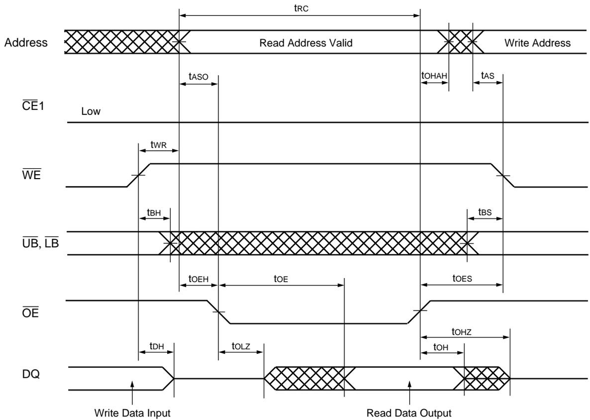
Note :  $\overline{CE1}$  can be tied to Low for  $\overline{WE}$  and  $\overline{OE}$  controlled operation.
