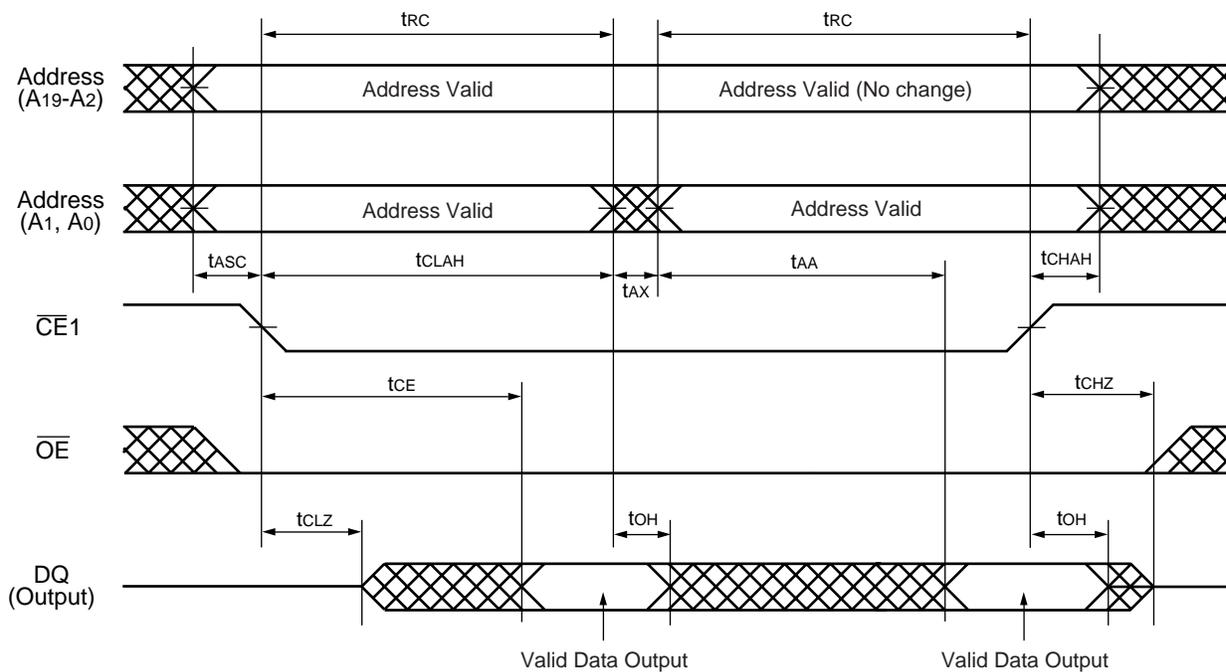
Note :  $\overline{CE2}$  and  $\overline{WE}$  must be High for entire read cycle.
