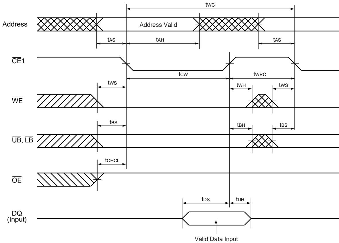
Note :  $\overline{CE2}$  must be High for write cycle.
