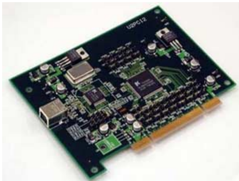
Figure 9-2 KL5KUSB201 PCI Evaluation Add-in Card
