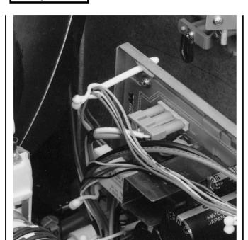
This connector can be connected to headers having 2.36mm diameter pins. Since the pitch between circuits is large, 8.0mm, this connector is ideally suited for the power supply circuits of TVs, stereo systems and VCRs.
