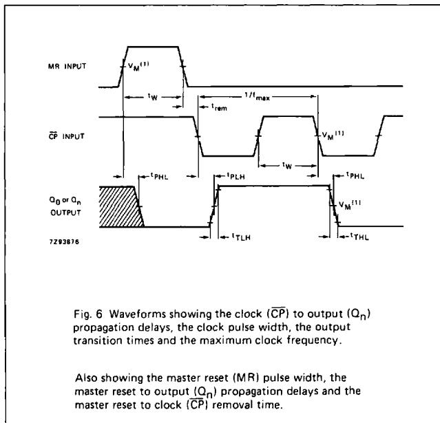
Fig. 6 Waveforms showing the clock ( $\bar{C}P$ ) to output ( $Q_n$ ) propagation delays, the clock pulse width, the output transition times and the maximum clock frequency.
