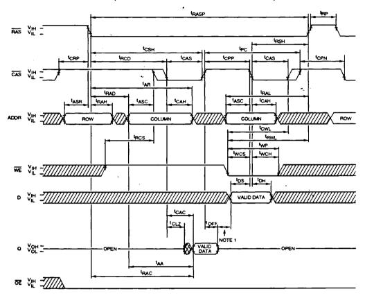
NOTE: 1. Do not drive data prior to High-Z; that is completion of <sup>t</sup>OFF. <sup>t</sup>CPP is equal to <sup>t</sup>OFF + <sup>t</sup>DS(MIN) + guardband between data-out and driving new data-in.
