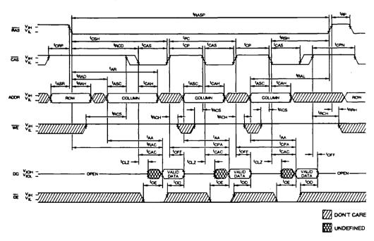
NOTE: 1. Applies to MT4C8513 L only; WE and DQ inputs on MT4C8512 L are "don't care" at RAS time. WE selects between normal WRITE and MASKED WRITE at RAS time. The DQ inputs are "don't care" for a normal WRITE (WE HIGH at RAS time). The DQ inputs provide the mask data at RAS time for a MASKED WRITE, WE LOW at RAS time.
