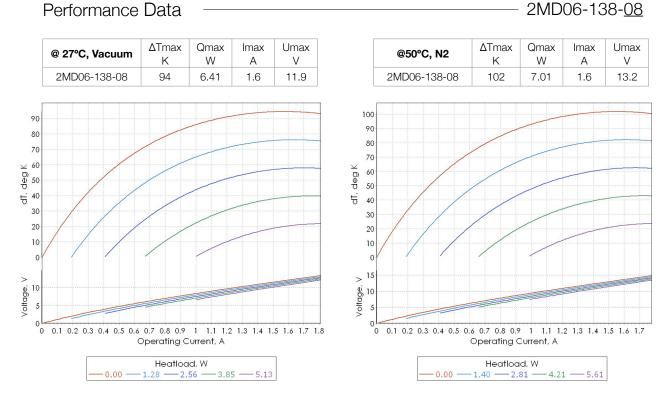
**Note**: Performance data is specified at optimal optimal conditions (TEC hot side is stabilized at ambient temperature). Any heatsink thermal resistance is not included into estimations. Use TECCad Software for estimations under different conditions.
