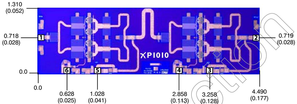
Units: millimeters (inches) Bond pad dimensions are shown to center of bond pad.
