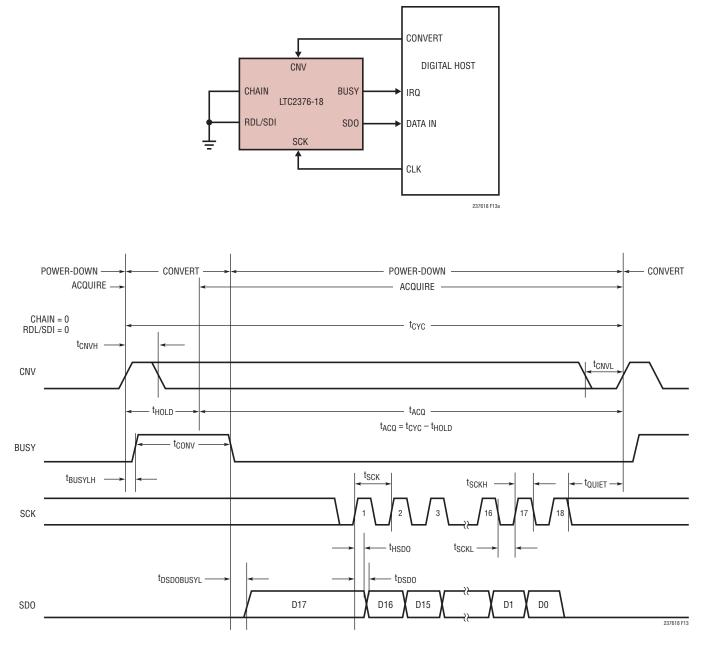
Figure 13. Using a Single LTC2376-18 in Normal Mode
