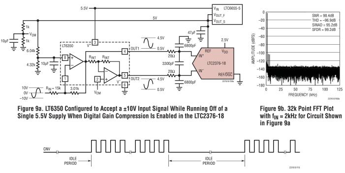
Figure 10. CNV Waveform Showing Burst Sampling
