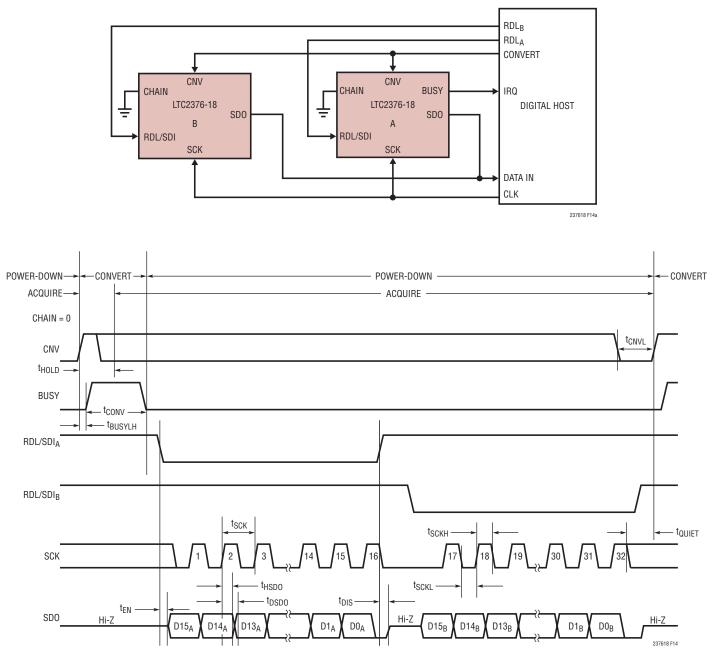
Figure 14. Normal Mode With Multiple Devices Sharing CNV, SCK and SDO
