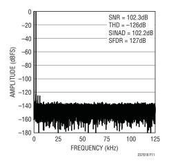
Figure 11. 32k Point FFT with  $f_{IN} = 2kHz$  of the LTC2376-18
