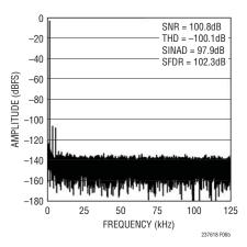
Figure 6b. 32k Point FFT Plot with  $f_{IN} = 2kHz$  for Circuit Shown in Figure 6a
