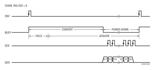
**Conversion Timing Using the Serial Interface**
