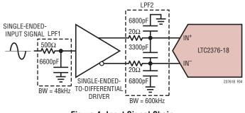
Figure 4. Input Signal Chain
