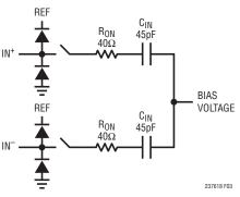
Figure 3. The Equivalent Circuit for the Differential Analog Input of the LTC2376-18
