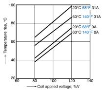
2. Ambient temperature characteristics and coil applied voltage
