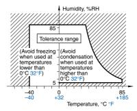
\* -40 to +85°C -40 to +185°F (When 45% to 80%V of coil holding voltage)
