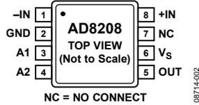
Figure 2. Pin Configuration
