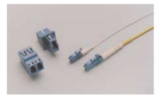
The LC connector was designed by Lucent Technology's Bell Labs. It is a small form factor connector based on the familiar RJ-45 telephone interface and is available in both simplex and duplex designs.
