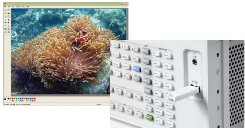
Figure 3. Availability of common PC interface offers an easy avenue to transfer customized patterns/images, EDID, firmware upgrade and Help files to and from USB flash drive.
