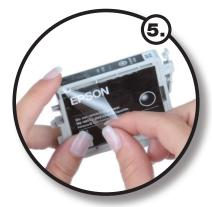
Seal the newly drilled hole with an adhesive strip and then leave the ink cartridge for a few hours to allow the ink enough time to spread throughout the ink chamber.
