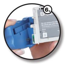
Finally, the ink cartridge chip ink fluid level reading needs to be reset. In order to do this, press the reset device (not included with the refill kit set) pins against the ink cartridge chip contact. After removing the adhesive tape from the ink outlet area, the refilled ink cartridge can then be inserted into the printer. Please be aware of the possibility of ink leakage.
