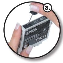
Next, using the tool provided, drill a hole approximately 7 mm deep through the designated opening. Drill carefully, as there are 2 inner walls to drill through.
