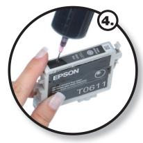
Now insert the syringe into the newly made opening and fill the ink chamber slowly and carefully until just below the opening. Should some of the ink leak out, simply remove it by using the syringe.
