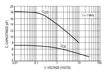
Figure 6. Capacitance versus Voltage
