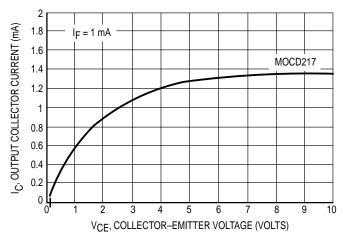
Figure 3. Output Current versus Collector–Emitter Voltage
