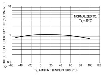
Figure 4. Output Current versus Ambient Temperature
