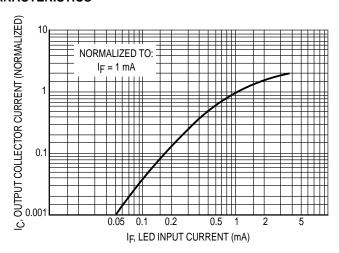
Figure 2. Output Current versus Input Current
