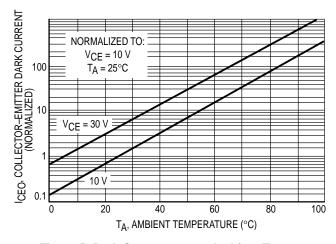
Figure 5. Dark Current versus Ambient Temperature
