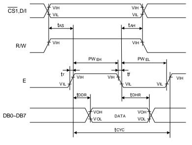
Fig.2 Read Operation Timing
