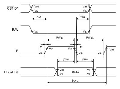
Fig.1 Write Operation Timing
