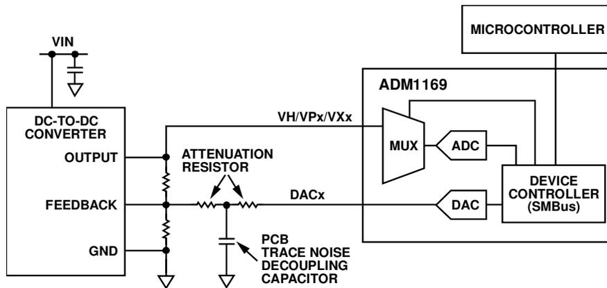
Figure 33. Closed-Loop Margining System Using the ADM1169
