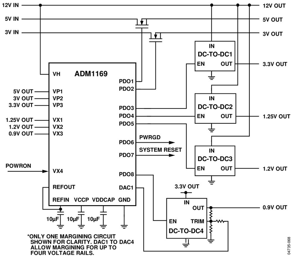
Figure 34. Applications Diagram
