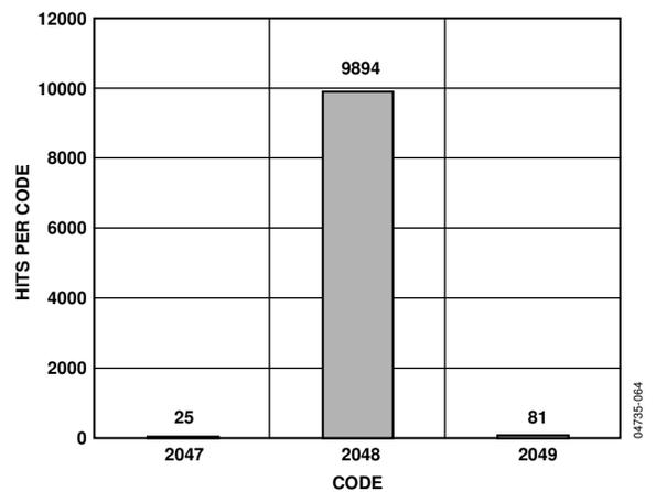
Figure 16. ADC Noise, Midcode Input, 10,000 Reads
