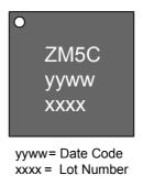
Figure 2: QFN Marking Information
