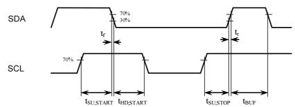
Figure 3: I2C Start and Stop timing
