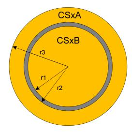
Figure 14: Typical SAR Capacitive Sensor
