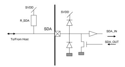
Figure 11: SDA Simplified Diagram
