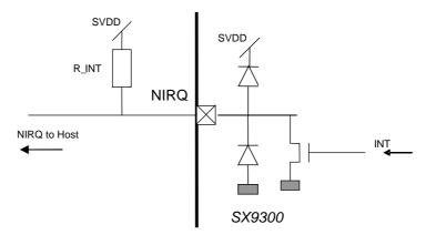
Figure 9: NIRQ Output Simplified Diagram
