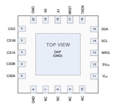
Figure 1: Pin Diagram
