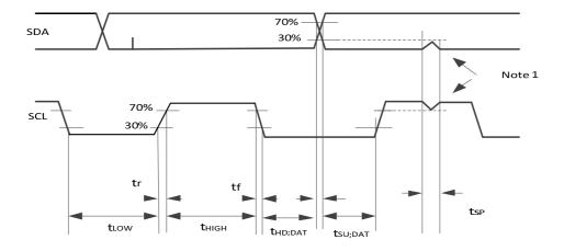
Figure 4: I2C Data timing
