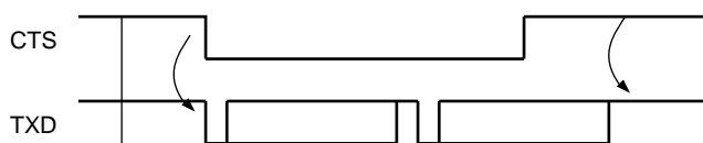
Figure 25-28. Transmitter Behavior when Operating with Hardware Handshaking
