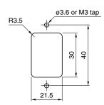
• Tighten the panel mounting M3 dia. bolt with the torque under 5.88X10<sup>-1</sup>N•m.
