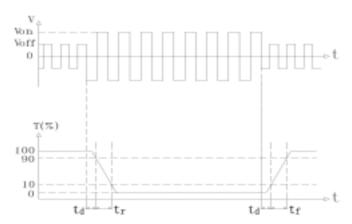
Turn on time:  $t_{on} = t_d + t_r$  Turn off time:  $t_{off} = t_d + t_f$  Measuring Condition:
