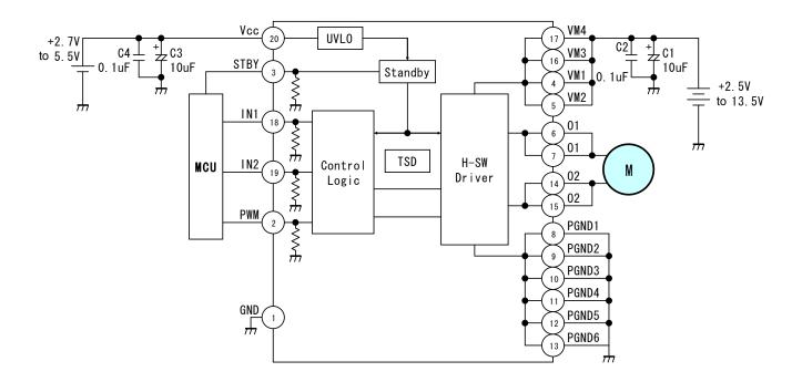
Note: Bypass capacitors (C1, C2, C3, and C4) should be connected as close as possible to the IC.
