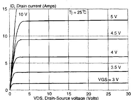
Fig. 5. Typical output characteristics.
