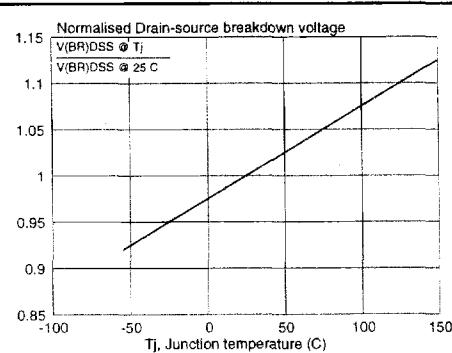
Fig.15. Normalised drain-source breakdown voltage.
