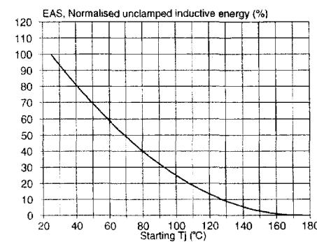
Fig.17. Normalised unclamped inductive energy.
