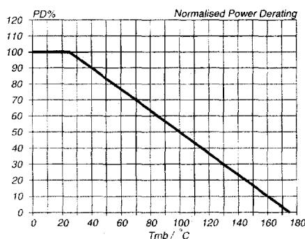
Fig. 1. Normalised power dissipation.
