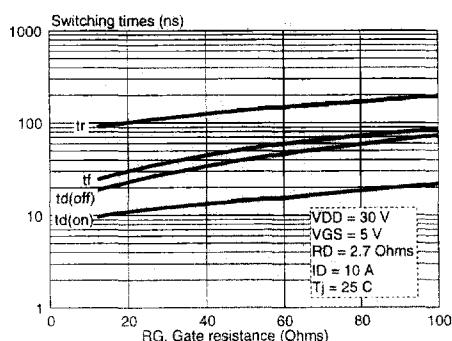
Fig.14. Typical switching times.
