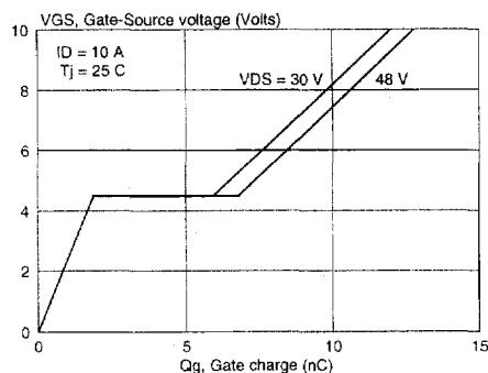
Fig.13. Typical turn-on gate-charge characteristics.
