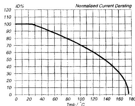
Fig. 2. Normalised continuous drain current.
