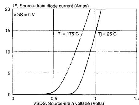
Fig.16. Source-Drain diode characteristic.
