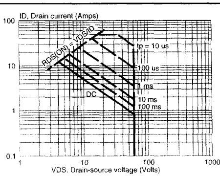
Fig. 3. Safe operating area.  $T_{mb} = 25^\circ C$
