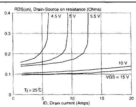
Fig. 6. Typical on-state resistance.
