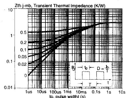
Fig. 4. Transient thermal impedance.
