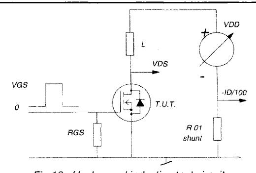
Fig.18. Unclamped inductive test circuit.
