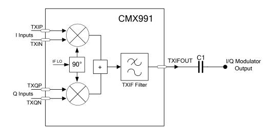
Figure 11 Example External Components - I/Q Modulator Output
