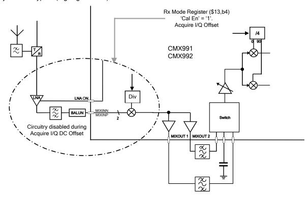
Figure 15 DC Offset Calibration Mode
