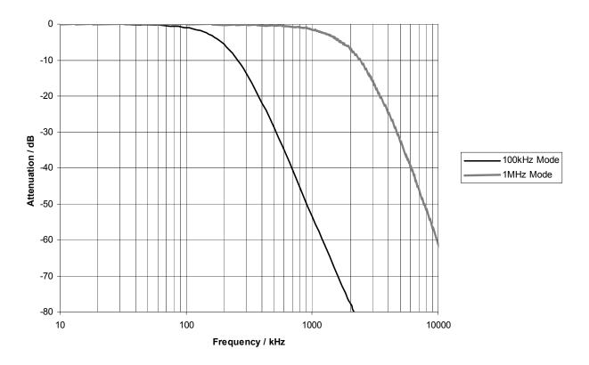
Figure 27 Typical Receiver I/Q Frequency Response
