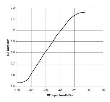
Figure 25 Typical SLI Performance in an Application Circuit (EV9920B) (Input 460MHz, 25kHz IF crystal filter: 45G15B1)
