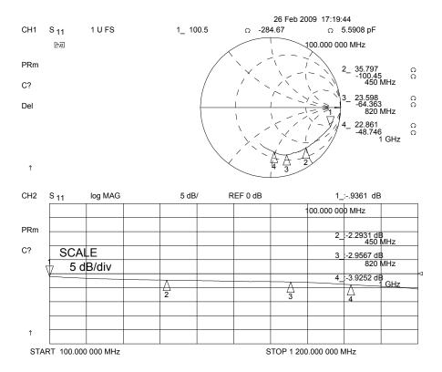
Figure 18 Typical LO Input Impedance
