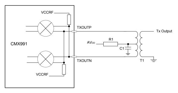
Figure 10 Example External Components - Transmitter
