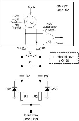
Figure 13 Example External Components - IF LO VCO External Tank Circuit
