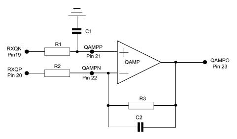
Figure 8 Example External Components - Receive I/Q Output
