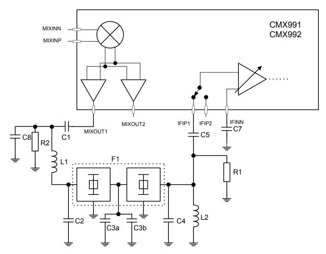
Figure 7 Example External Components – Receive 1st IF Section
