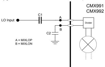
Figure 12 Example External Components – Rx LO Input
