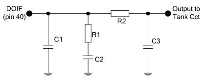
Figure 14 Example External Components - IF LO Loop Filter
