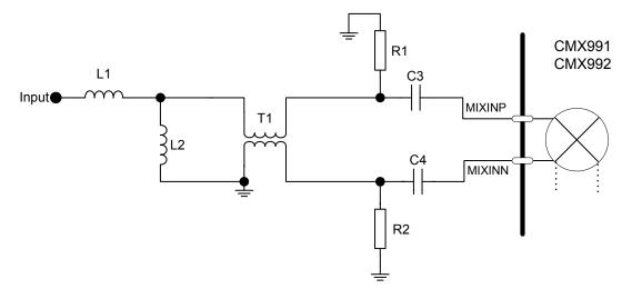
Figure 6 Example External Components – Receive 1<sup>st</sup> Mixer Input
