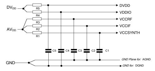
Figure 5 Recommended Power Supply Connections and Decoupling
