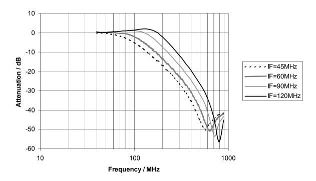
Figure 29 Transmitter Path IF Filters
