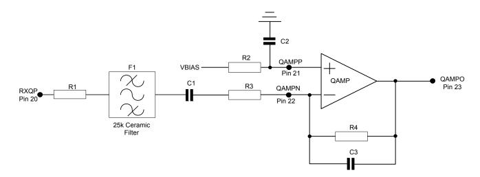
Figure 9 Example External Components - Receive Low IF Output
