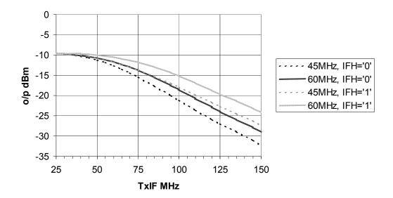
Figure 31 Effect of IFH on 45MHz and 60MHz Transmitter IF Filters
