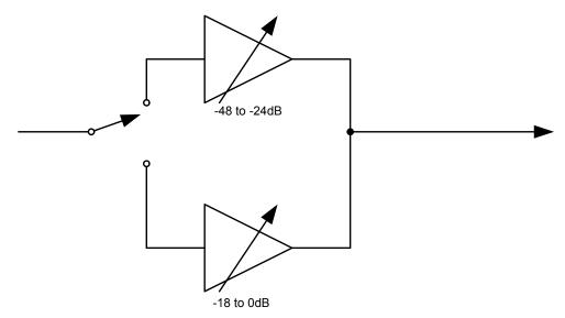
Figure 20 Receiver Gain Control
