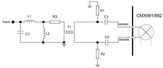
**Figure 21 Receiver Matching Components**
