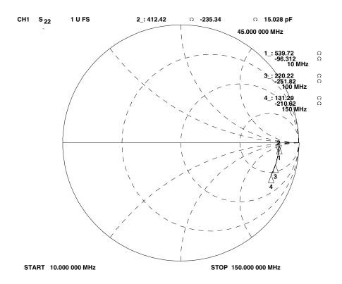
Figure 22 MIXOUT1 Port Impedance (unmatched)
