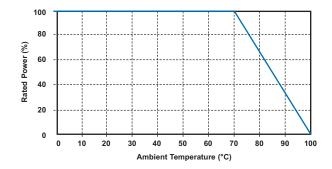
When the ambient temperature exceeds 70°C, reduce the rated power and current in accordance with the derating curve given
