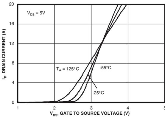
Figure 5. Transfer Characteristics.
