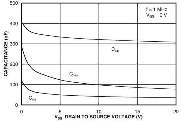
Figure 8. Capacitance Characteristics.
