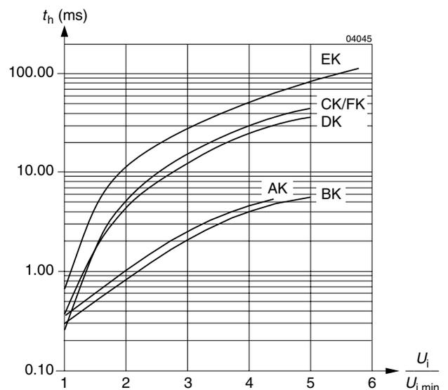
Fig. 6 Typical hold-up time  $t_h$  versus relative input voltage  $U_i/U_{i min}$ . The DC-DC converters require an external series diode in the input path if other loads are connected to the same input supply lines.
