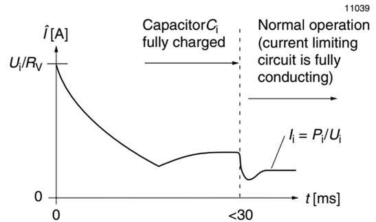
$R_V$ : Current limiting resistance =  $R_S + R_I = 15 \Omega$
