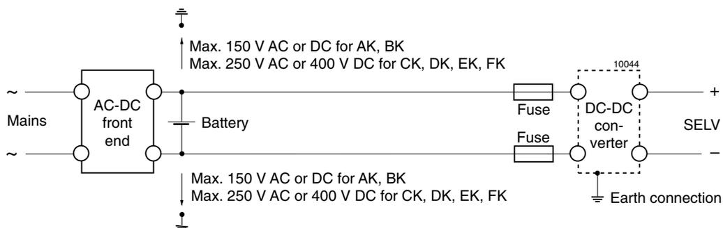
Fig. 24 Schematic safety concept. Use earth connection as per table: Safety concept leading to an SELV output circuit. Use fuse if required by the application. See also: *Installation Instructions*.
