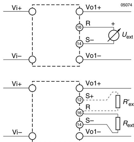
Fig. 16 Output voltage control for single output units AK...EK 1000 by means of the R input
