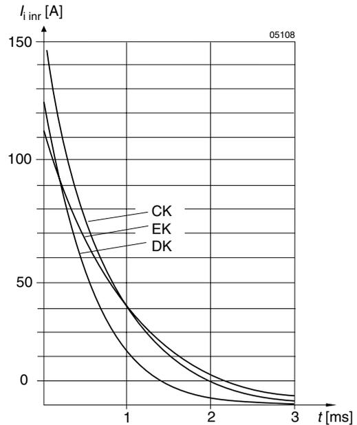
Fig. 5 Typical inrush current versus time at  $U_{i max}$ ,  $R_{ext} = 0$ . For AK, BK and FK as well as for application related values use the formula given in Inrush Current Peak Value to get realistic results.
