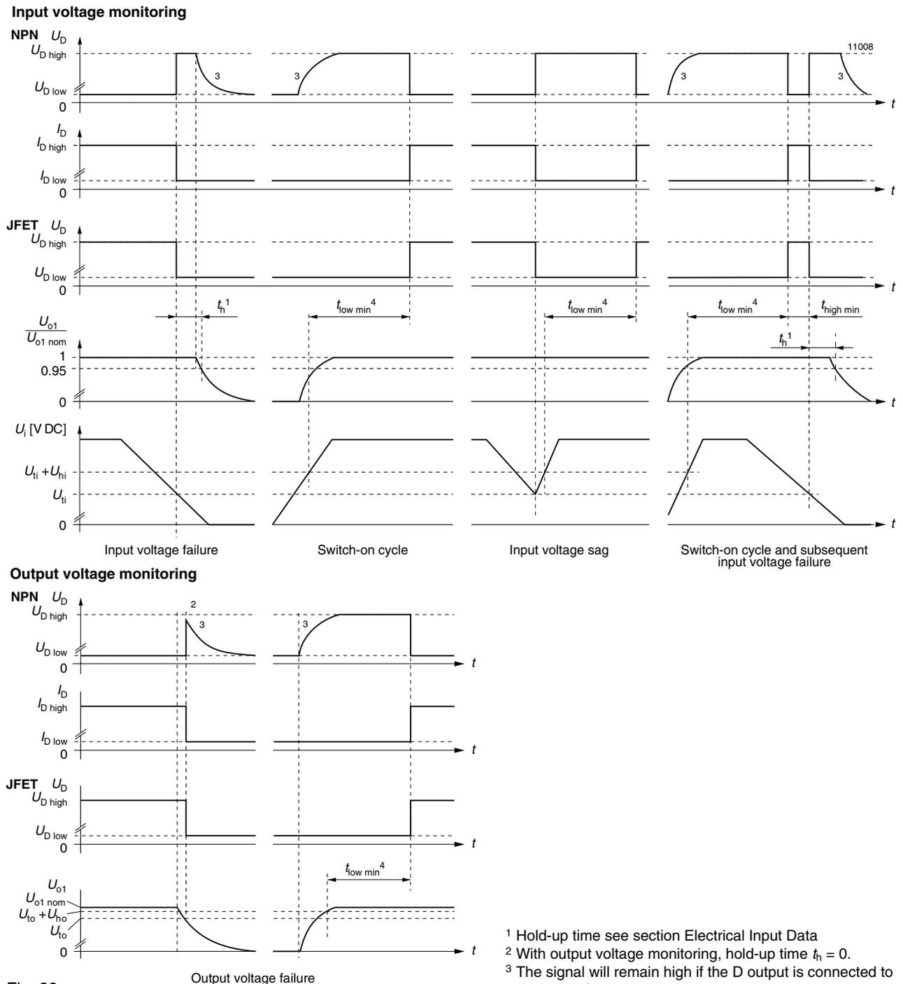
Fig. 33 Relationship between  $U_i$ ,  $U_{o1}$ ,  $U_D$ ,  $U_{o1}/U_{o\ nom}$  versus time
