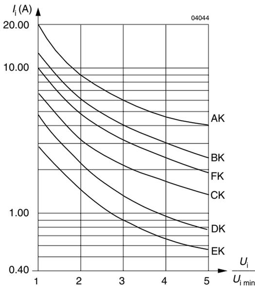
Fig. 3 Typical input current versus relative input voltage
