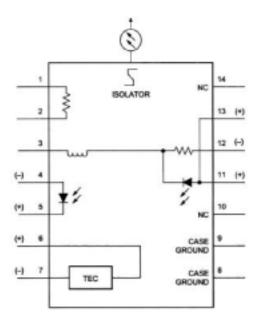
Figure 1. 1754W Laser Schematic
