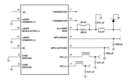
Figure 2. 1754W Circuit Schematic
