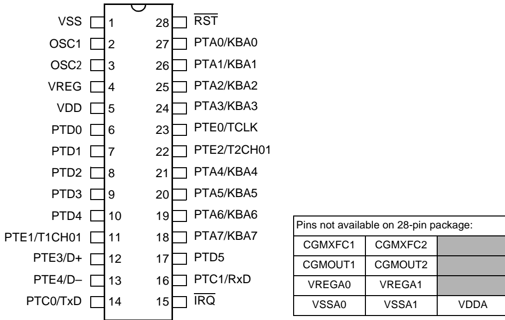
Figure 1-3. 28-Pin SOIC Pin Assignment
