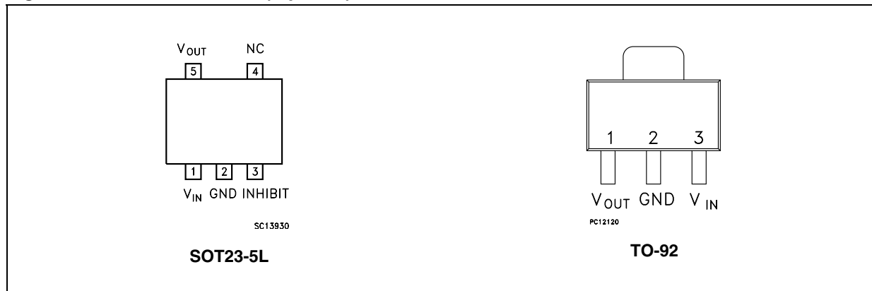
Figure 2. Pin connections (top view)
