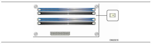
Figure 7. Location of the Standby Power Indicator LED
