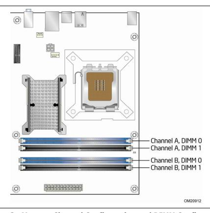
Figure 3. Memory Channel Configuration and DIMM Configuration
