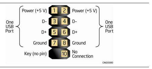
Figure 12. Connection Diagram for Front Panel USB Headers
