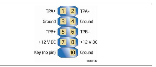
Figure 13. Connection Diagram for IEEE 1394a Header
