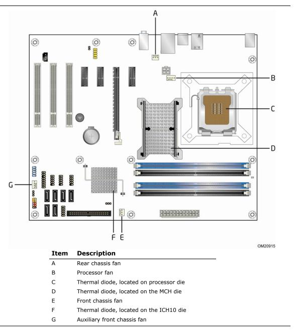
Figure 6. Thermal Sensors and Fan Headers
