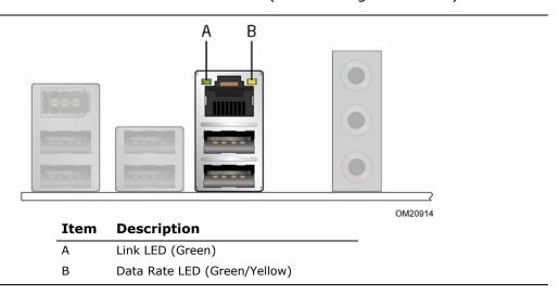
Figure 5. LAN Connector LED Locations
