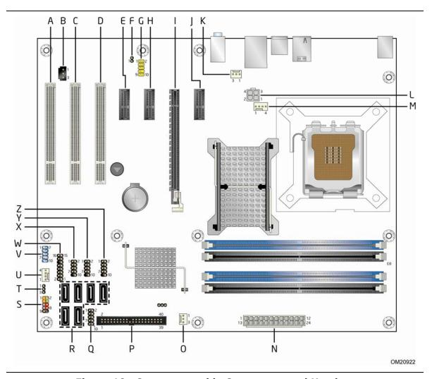
Figure 10. Component-side Connectors and Headers
