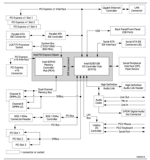
Figure 2. Block Diagram
