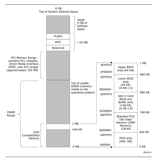
Figure 8. Detailed System Memory Address Map
