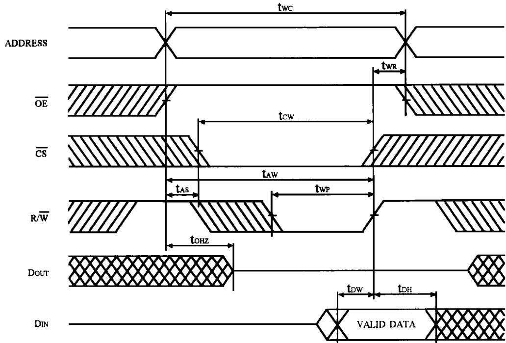
WRITE CYCLE 3 ( $\overline{\text{CS}}$  CONTROL,  $\overline{\text{OE}} = \text{LOW}$ )
