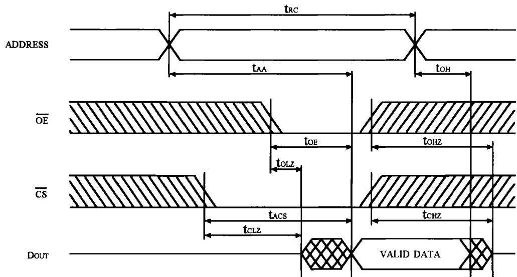
**READ CYCLE 2 ( $R/W$  CONTROL,  $\overline{OE} = LOW$ ,  $\overline{CS} = LOW$ )**
