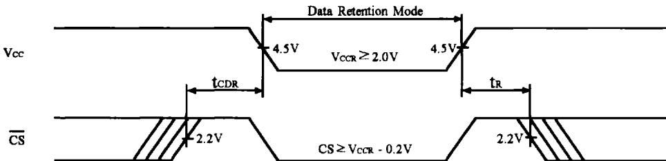
\*Note: When retaining data in standby mode, supply voltage can be lowered within a certain range.
