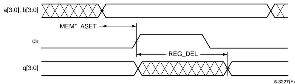
**Figure 57. Read Operation—LUT Memory Loading Flip-Flops**
