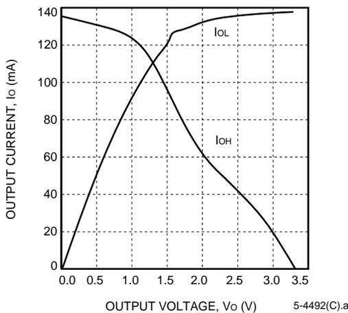
**Figure 86. Fast ( $T_J = 25\text{ }^\circ\text{C}$ ,  $V_{DD} = 3.3\text{ V}$ )**
