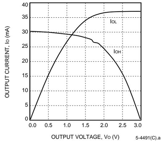
**Figure 87. Sinklim ( $T_J = 125\text{ }^\circ\text{C}$ ,  $V_{DD} = 3.0\text{ V}$ )**
