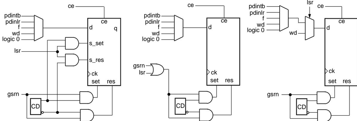
A. Latch/FF with Local Synchronous Set or Reset
