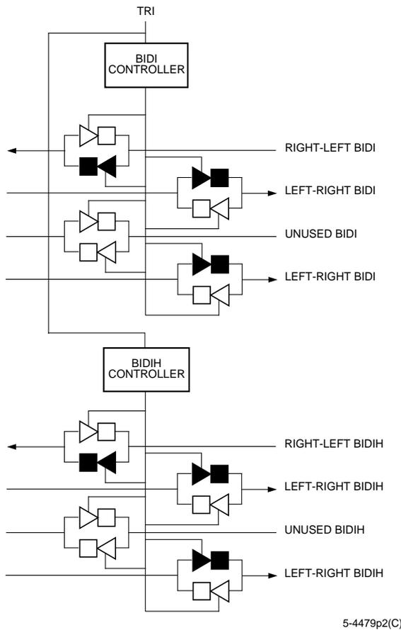
Figure 20. 3-Statable Bidirectional Buffers
