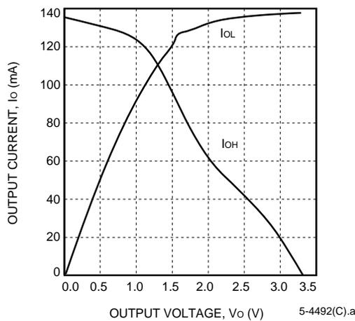
**Figure 85. Slewlim ( $T_J = 25\text{ }^\circ\text{C}$ ,  $V_{DD} = 3.3\text{ V}$ )**
