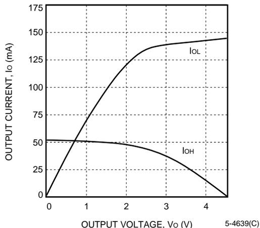
Figure 83. Fast ( $T_J = 125\text{ }^\circ\text{C}$ ,  $V_{DD} = 4.5\text{ V}$ )
