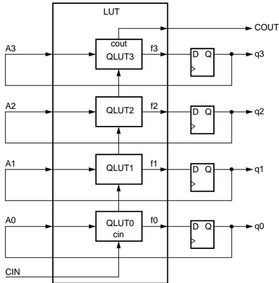
Figure 10. Counter Submode with Flip-Flops
