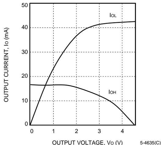
Figure 81. Sinklim ( $T_J = 125\text{ }^\circ\text{C}$ ,  $V_{DD} = 4.5\text{ V}$ )
