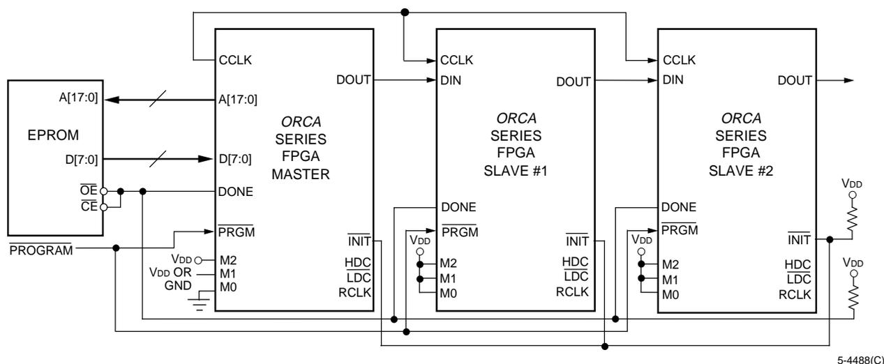
Figure 47. Daisy-Chain Configuration Schematic
