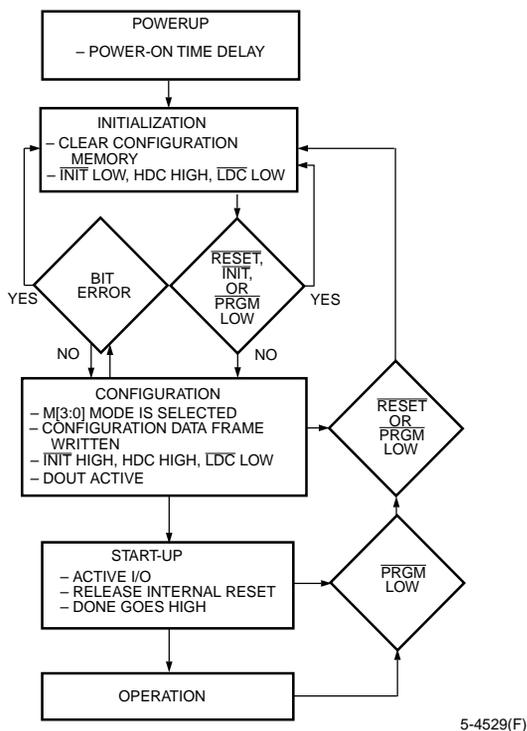
Figure 36. FPGA States of Operation
