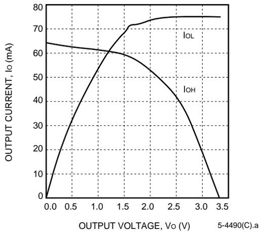
**Figure 84. Sinklim ( $T_J = 25\text{ }^\circ\text{C}$ ,  $V_{DD} = 3.3\text{ V}$ )**
