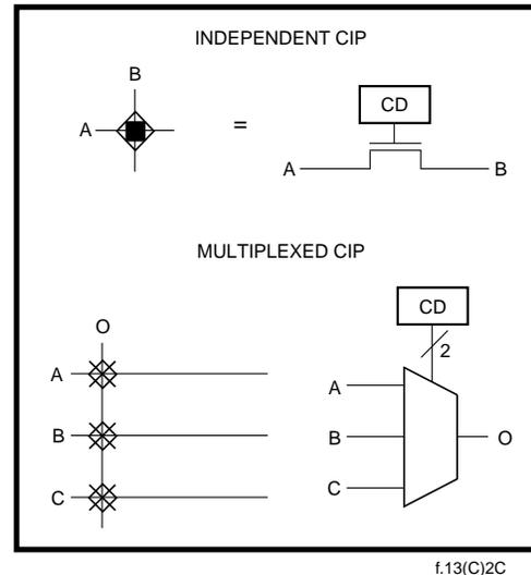
Figure 19. Configurable Interconnect Point
