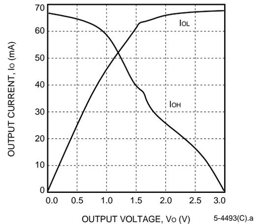
**Figure 89. Fast ( $T_J = 125\text{ }^\circ\text{C}$ ,  $V_{DD} = 3.0\text{ V}$ )**
