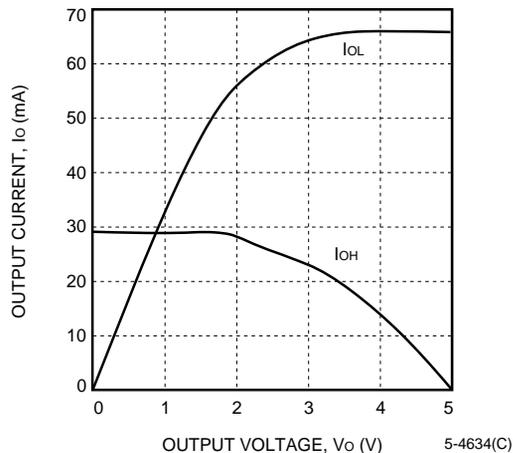
Figure 78. Sinklim ( $T_J = 25\text{ }^\circ\text{C}$ ,  $V_{DD} = 5.0\text{ V}$ )
