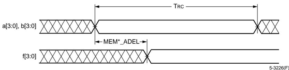
**Figure 56. Read Operation—Flip-Flop Bypass**
