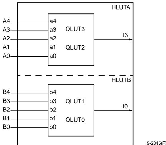
**Figure 5. F5 Mode—Two Functions of Five Input Variables**
