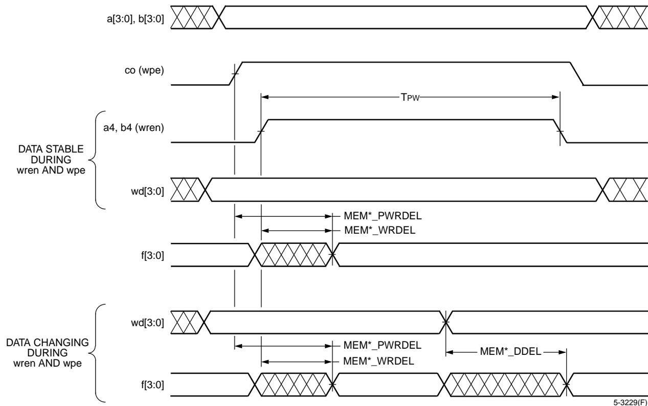
Figure 59. Read During Write
