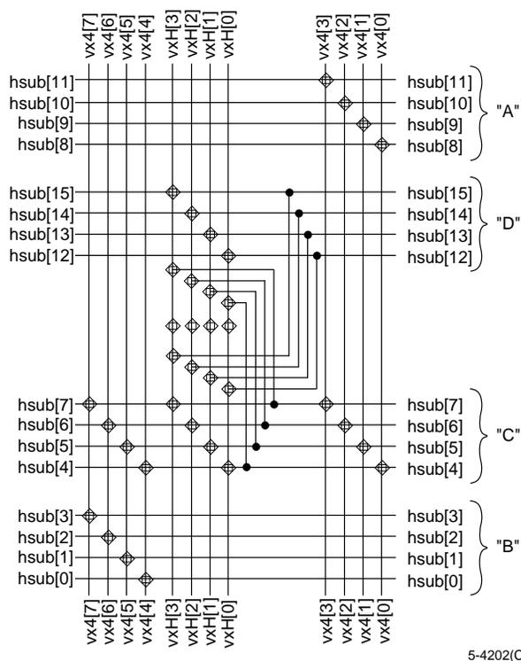
**Figure 32. Horizontal Subquad Routing Connectivity (Half Quad)**
