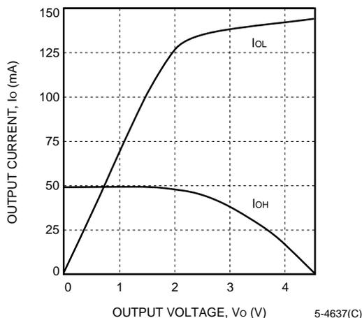
Figure 82. Slewlim ( $T_J = 125\text{ }^\circ\text{C}$ ,  $V_{DD} = 4.5\text{ V}$ )
