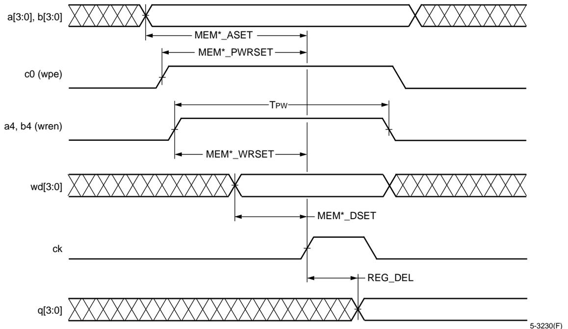
Figure 60. Read During Write—Clocking Data into Flip-Flop
