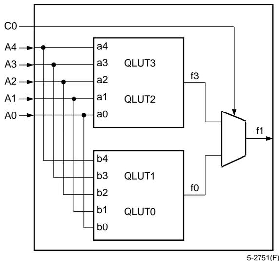
**Figure 8. F5M Mode—One Six-Input Variable Function**
