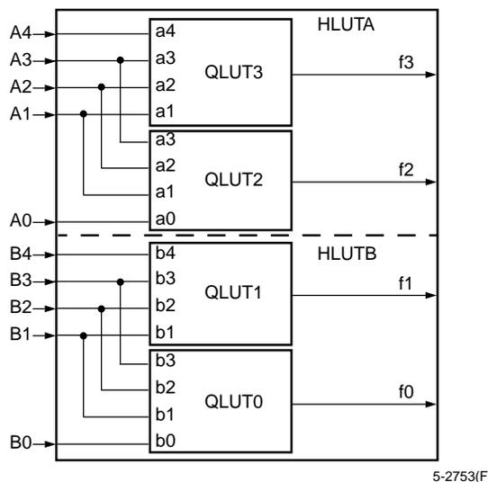
**Figure 4. F4 Mode—Four Functions of Four Input Variables**
