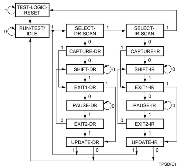
Figure 51. TAP Controller State Transition Diagram
