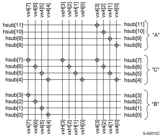
**Figure 31. Horizontal Subquad Routing Connectivity**
