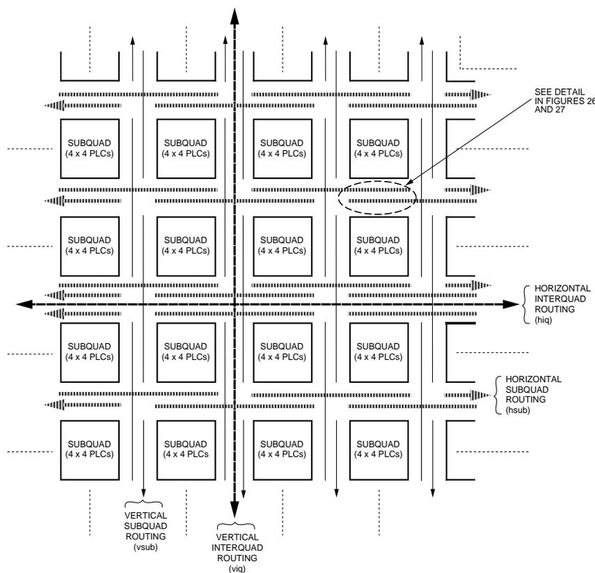
Figure 30. Subquad Blocks and Subquad Routing
