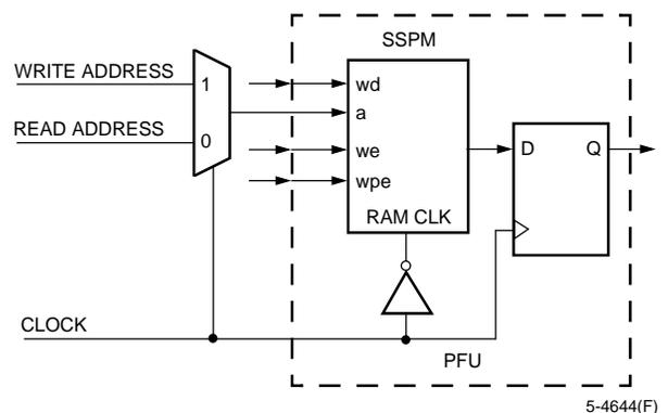
Figure 15. SSPM with Read/Write per Clock Cycle
