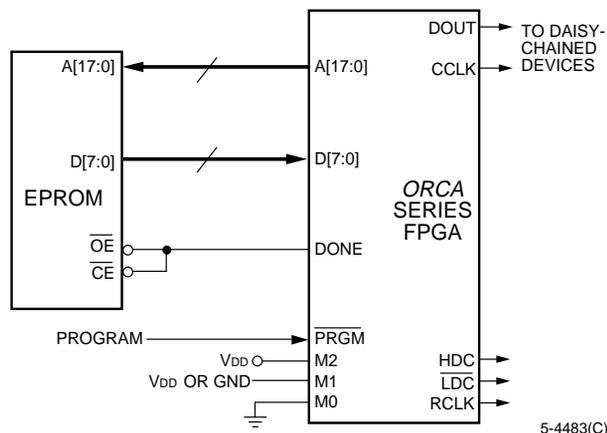
Figure 41. Master Parallel Configuration Schematic
