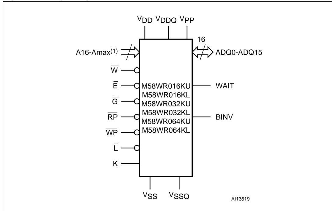
1. Amax is equal to A19 in the M58WR016KU/L, to A20 in the M58WR032KU/L, and to A21 in the M58WR064KU/L.
