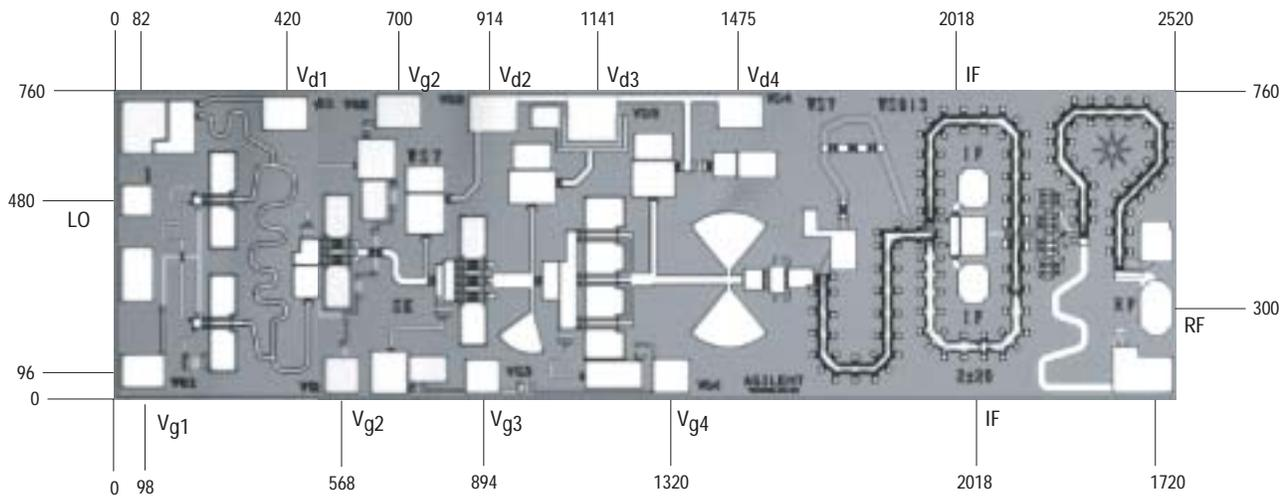
Figure 15. AMMC-3040 Bond Pad Locations, dimensions in microns.
