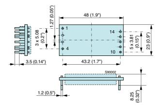
Fig. 3 Open frame Weight: <20 g
