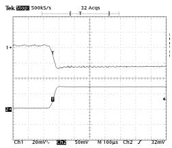
Operating conditions are as follows: Vin=5V, Vo=3.3V, Load change from Io=100% to Io=0%, TA=25°C, Cin=0F, Co= $\mu$ F.
