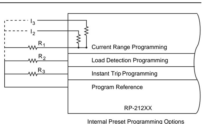
**FIGURE 3. RP-212XX SERIES PROGRAMMING CONNECTIONS**
