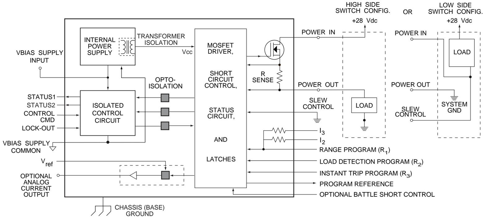
FIGURE 1. STAR Series BLOCK DIAGRAM
