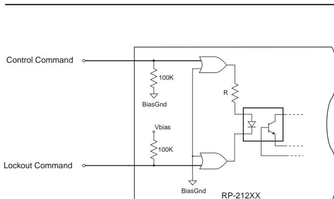
**FIGURE 2. RP-212XX SERIES CONTROL/LOCKOUT FUNCTIONAL SCHEMATIC**
