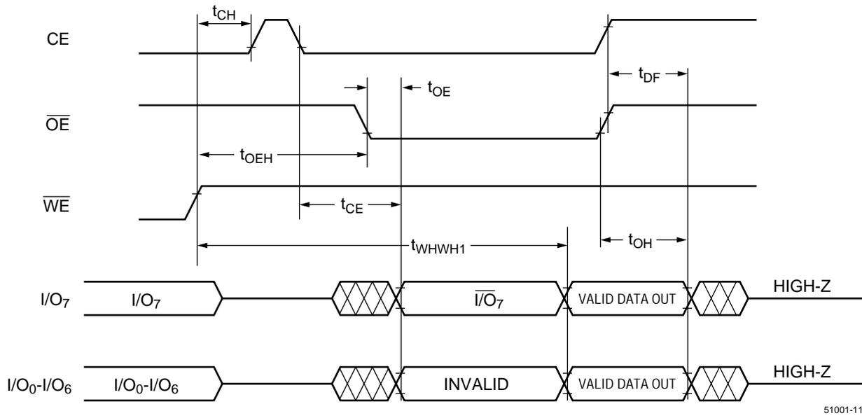
**Waveforms of Toggle Bit Cycle**
