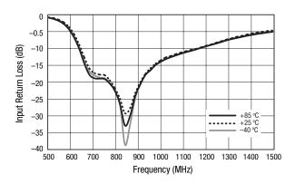
Figure 5. Input Return Loss vs Frequency Over Temperature,  $P_{\text{IN}} = -20 \text{ dBm}$
