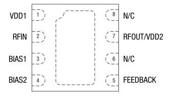
Figure 2. SKY65037-360LF Pinout – 8-Pin QFN (Top View)
