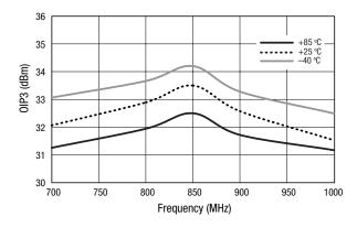
Figure 8. OIP3 vs Frequency Over Temperature, PIN = -18 dBm/Tone, 5 MHz Tone Spacing
