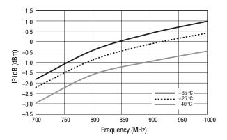
Figure 9. IP1dB vs Frequency Over Temperature
