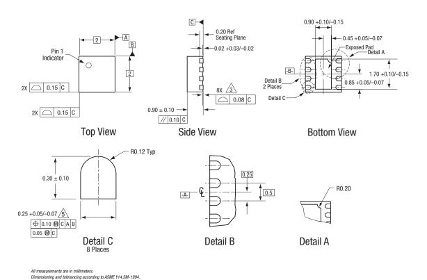
Figure 13. SKY65037-360LF 8-Pin QFN Package Dimensions
