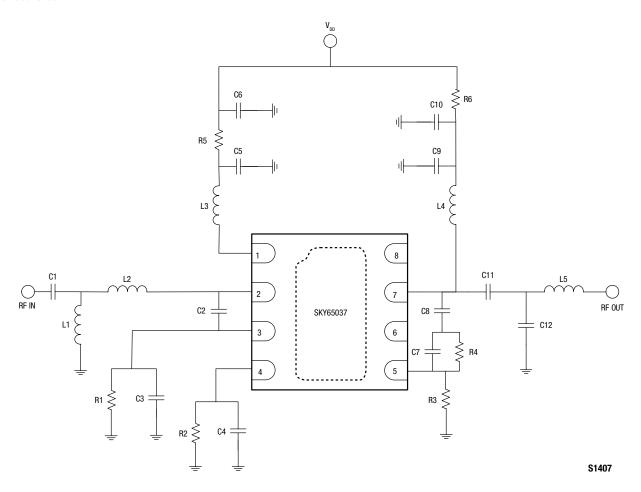
Figure 11. SKY65037-360LF Evaluation Board Schematic
