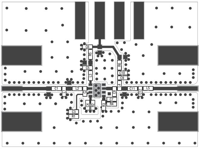
C1, C2, L1, and L2 comprise the input matching network C11, C12, and L5 comprise the output matching network.
