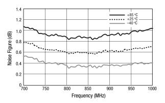
Figure 6. Noise Figure vs Frequency Over Temperature, Input RF Connector and Board Trace De-Embedded From Measurement
