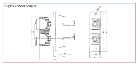
Standard split sleeve for single mode is zirconia and for multimode phosphor bronze.
