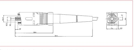
Standard ferrule for single mode and for multimode is zirconia. Polymer ferrules for multimode on request. Standard ferrule hole diameter is 126  $\mu$ m. For other diameters, consult FCI. Cable sizes are standard 2.4 to 3.0 mm.
