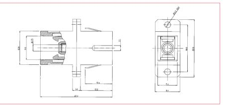
Standard split sleeve for single mode is zirconia and for multimode phosphor bronze.
