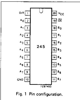
Fig. 1 Pin configuration.
