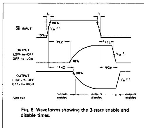
Fig. 6 Waveforms showing the 3-state enable and disable times.
