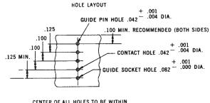
CENTER OF ALL HOLES TO BE WITHIN ,006" DIAMETER OF TRUE POSITION.
